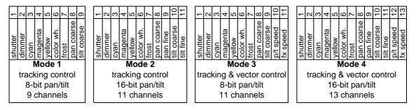
The DMX modes are summarized above. Mode 4 provides full control; it is recommended unless channels are limited.
