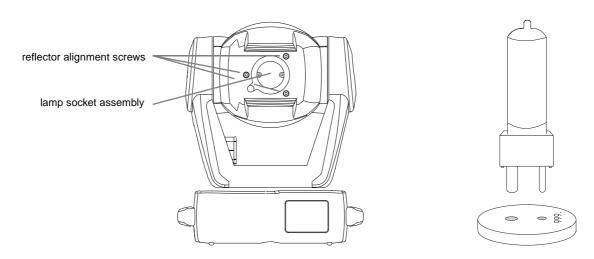
Figure 1: Lamp installation
