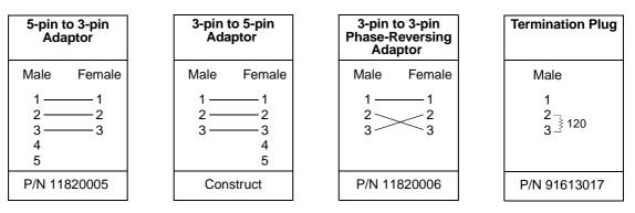
Figure 2: Cable adaptors and termination
